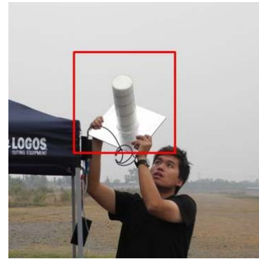
Figure 10 Receiver of 900 MHz omnidirectional transmission antenna on the ground
