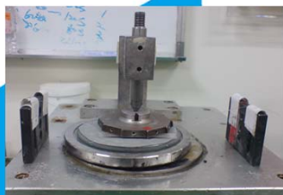
Grinding machine for Optical Fiber Profile of the D-shaped polished fiber The SEM and AFM micrographs of gratings Optical spectrum of our Novel Optical Wavelength Filter
