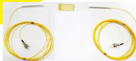
The Co-60 source gamma-ray irradiation instrument and Schematic diagram The Novel Optical Wavelength Filter The reflected optical wavelength ( \lambda ) varies with the surrounding temperature( ^{\circ}\text{C} )
